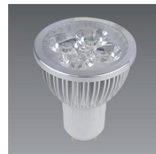
Item No: CSL-3603 Lamp power: 4x1W Base: GU10 Color: R/G/B/Y/W/WW Working voltage: DC/AC 230V Materials: Aluminum+lens
