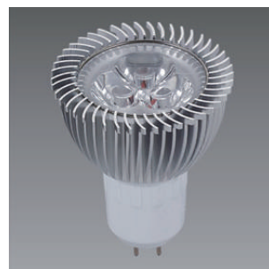
Item No: CSL-3502 Lamp power: 1x3W/3x1W Base: G5.3 Color: R/G/B/Y/W/WW Working voltage: DC/AC 230V Materials: Aluminum+lens
