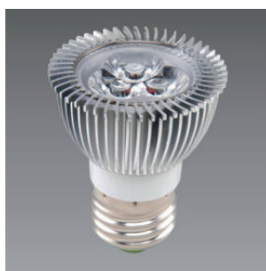
Item No: CSL-3504 Lamp power: 1x3W/3x1W Base: E27 Color: R/G/B/Y/W/WW Working voltage: DC/AC 230V Materials: Aluminum+lens
