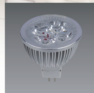
Item No: CSL-3601 Lamp power: 4x1W Base: MR16 Color: R/G/B/Y/W/WW Working voltage: DC/AC 12V Materials: Aluminum+lens
