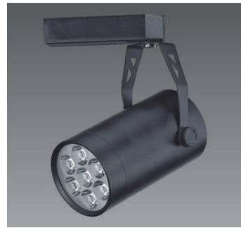
CSL-4203 Lamp power: 7x1W Color: R/G/B/Y/W/WW Working voltage: DC/AC 230V Materials: Aluminum+lens
